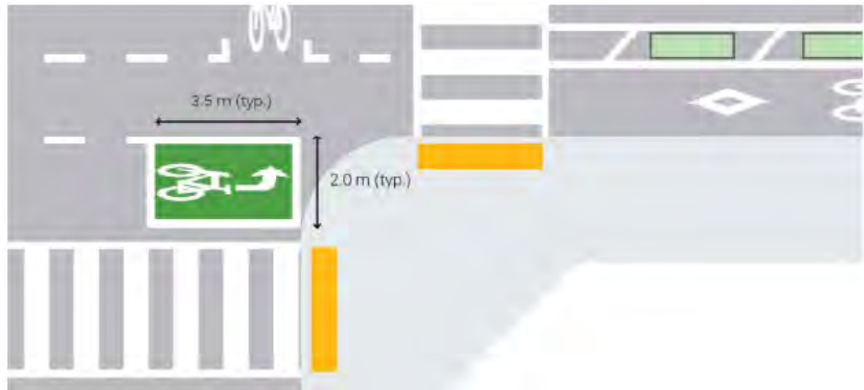
Figure 5.12: On-street two-stage queue box detail (Source: OTM Book 18)
