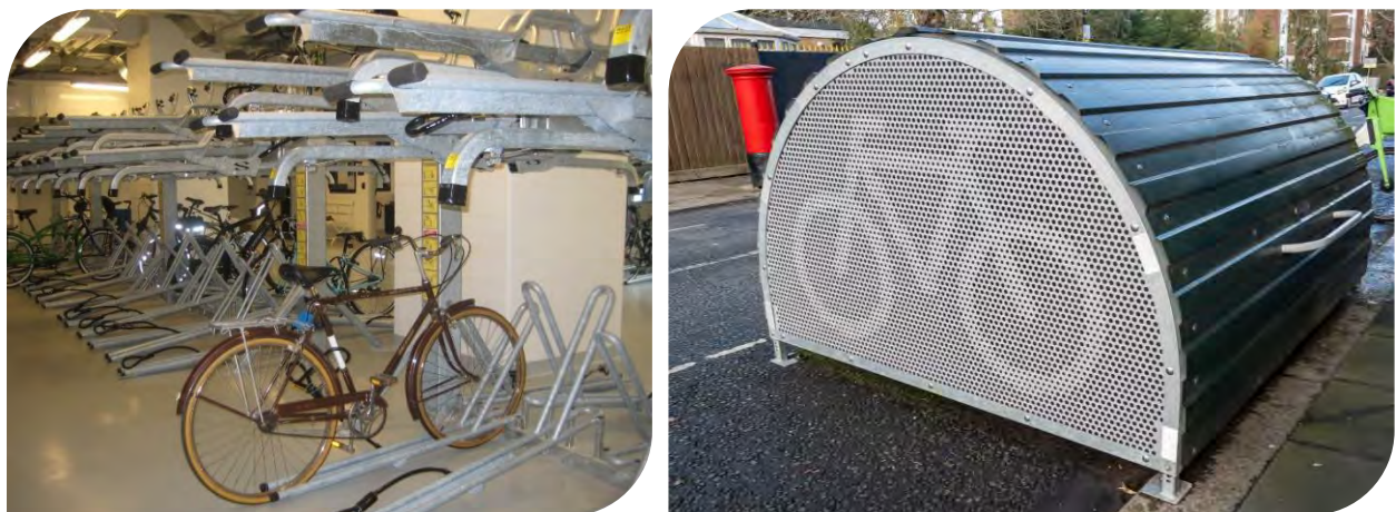
Figure 6.12: Example of long-term bike parking, including stacked bicycle parking (left) and bike lockers (right)
