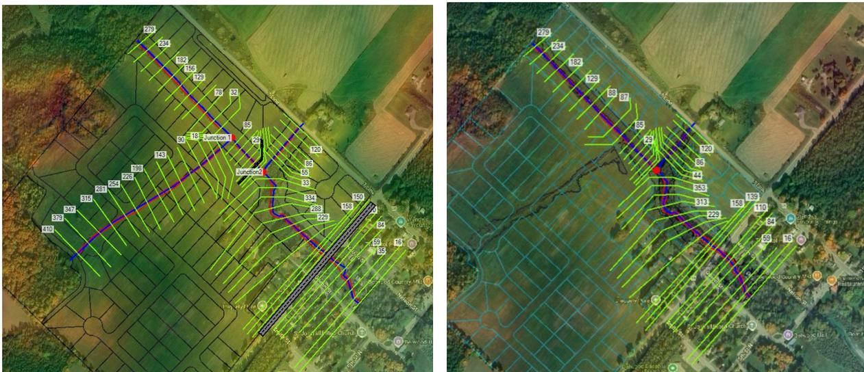
**Figure 5.3: Hydraulic Model Set Up Existing (Left) vs Proposed (Right)**
