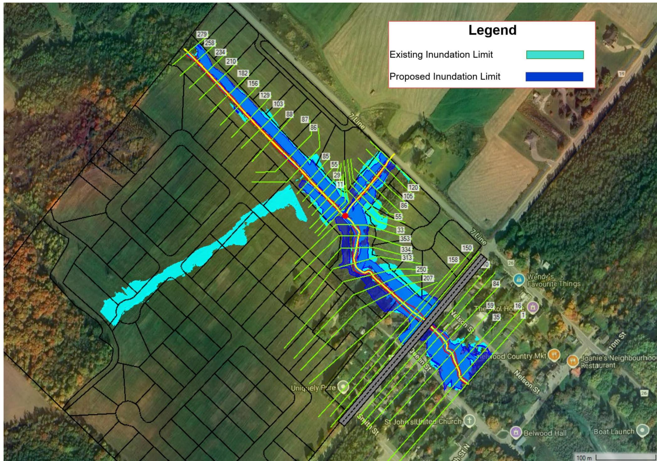
**Figure 5.5: 12-hour Regional Storm Event Inundation Boundaries for Existing vs Proposed**
